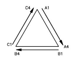
NOTE: ALPHA STARTS AT Q (NORTH) OR FIRST AZIMUTH AFTER Q NOTE: ALPHA STARTS AT U (NORTH) OR FIRST AZIMUTH AFTER O NOTE: BETA IS FIRST AZIMUTH AFTER ALPHA IN CLOCK-WISE DIRECTION NOTE: GAMMA IS FIRST AZIMUTH AFTER GAMMA IN CLOCK-WISE DIRECTION NOTE: AZIMUTH IS IDENTIFIED BY THE PANEL, NOT THE ELEMENTS INSIDE
