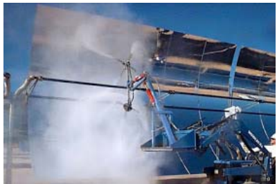
Sandia National Laboratory Mr Twister mirror washing machine is the most cost-effective
