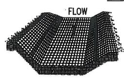
IN DITCHES, APPLY PROTECTIVE COVERING PARALLEL TO THE DIRECTION OF FLOW. AVOID JOINING MATERIAL IN THE CENTER OF THE DITCH IF AT ALL POSSIBLE.
