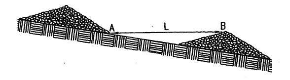
L = DISTANCE SUCH THAT POINTS A AND B ARE OF EQUAL ELEVATION.
