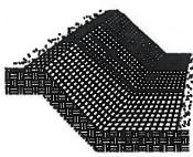
ON STEEP SLOPES, APPLY PROTECTIVE COVERING PERPENDICULAR TO THE DIRECTION OF FLOW AND ANCHOR SECURELY.
