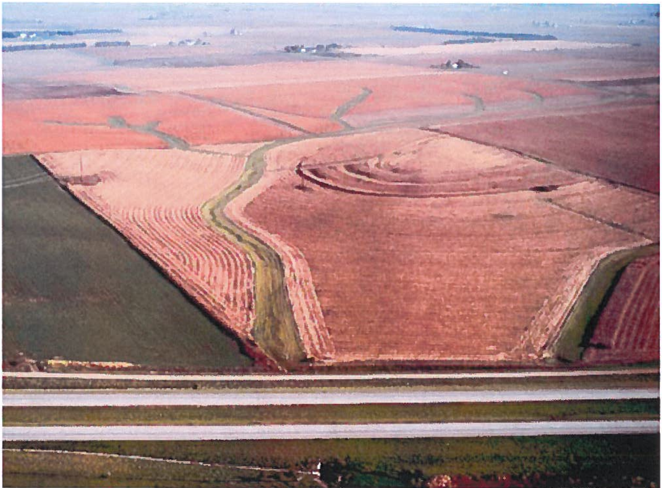
Figure 5.—A combination of grassed waterways and narrow-based terraces helps to prevent further erosion in an area of Wyonet silt loam, 5 to 10 percent slopes, eroded.
