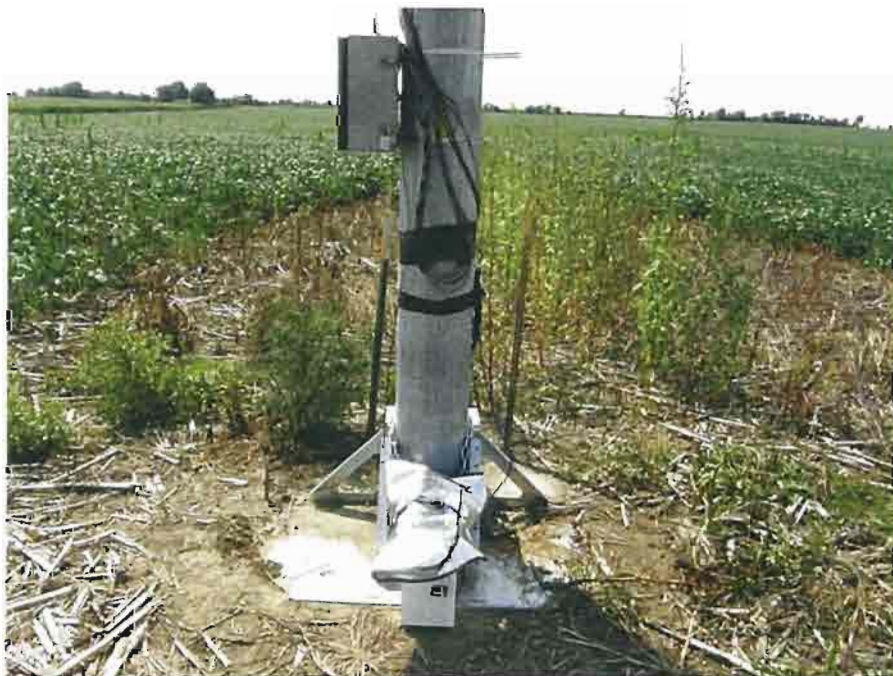
Photo 9. MET Tower 3 (9129) ground set-up covered with solar reflector to prevent overheating.
