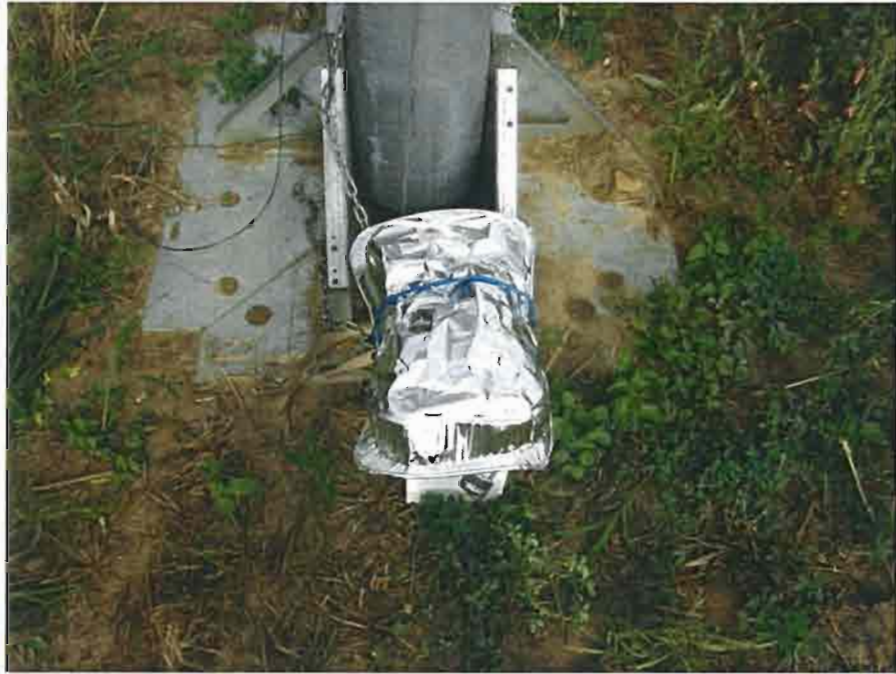
Photo 8. MET Tower 1 (9128) ground set-up covered with solar reflector to prevent overheating.
