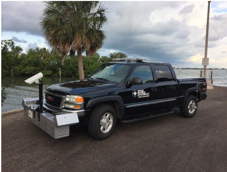
Figure 1. ARA collects high-resolution digital images and roughness data for Champaign County's highways using an automated digital survey vehicle.
