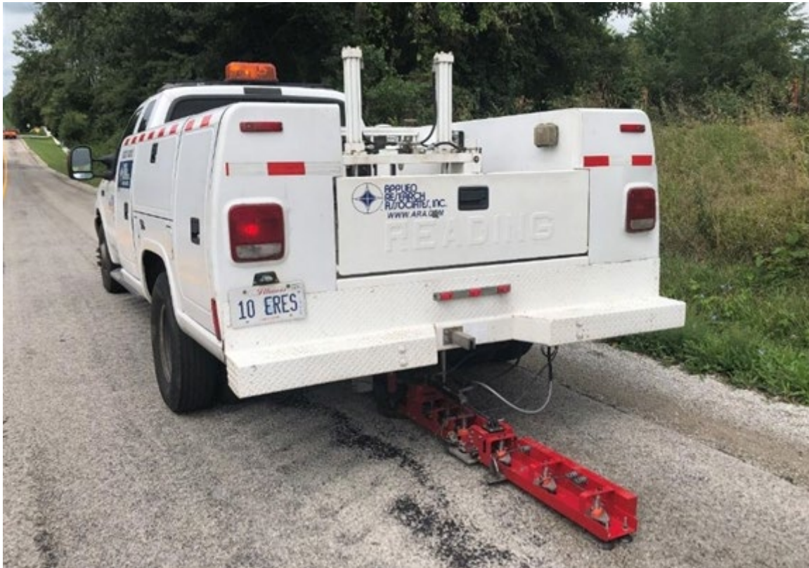
Figure 3. ARA performs structural evaluation with a JILS truck-mounted FWD.
