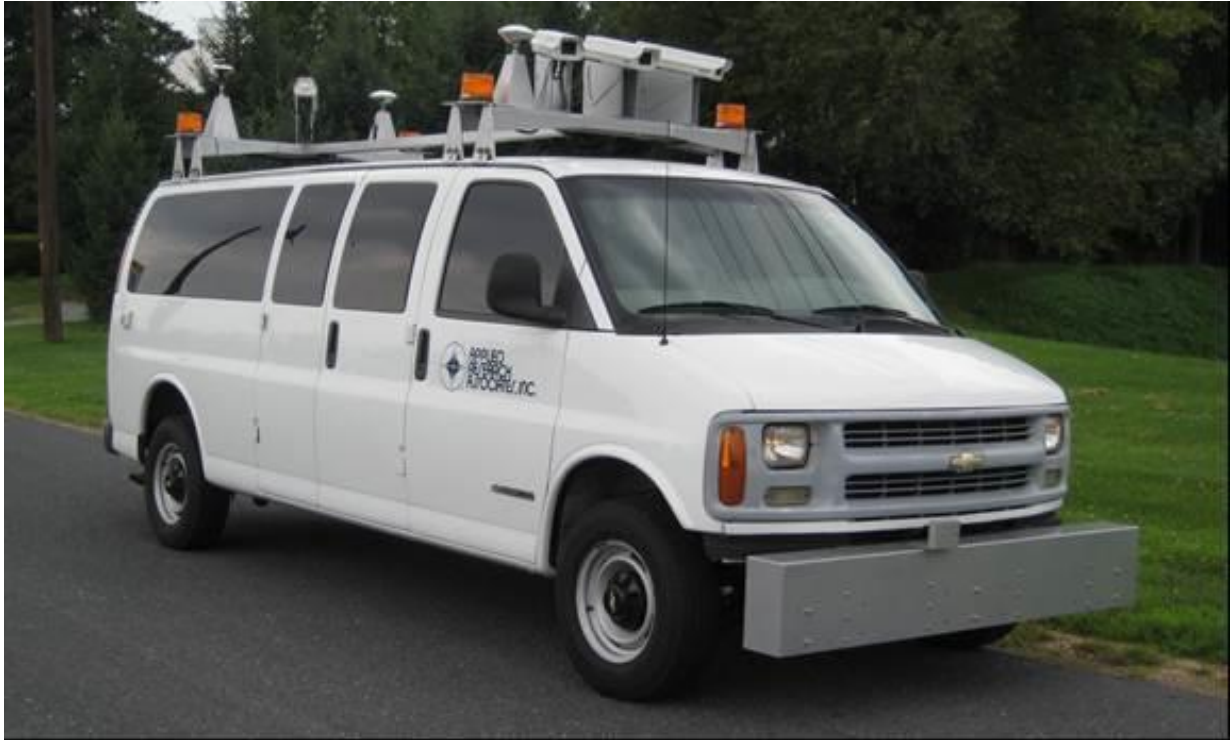
Figure 1. ARA collects high-resolution digital images and roughness data for Champaign County's highways using an automated digital survey vehicle.
