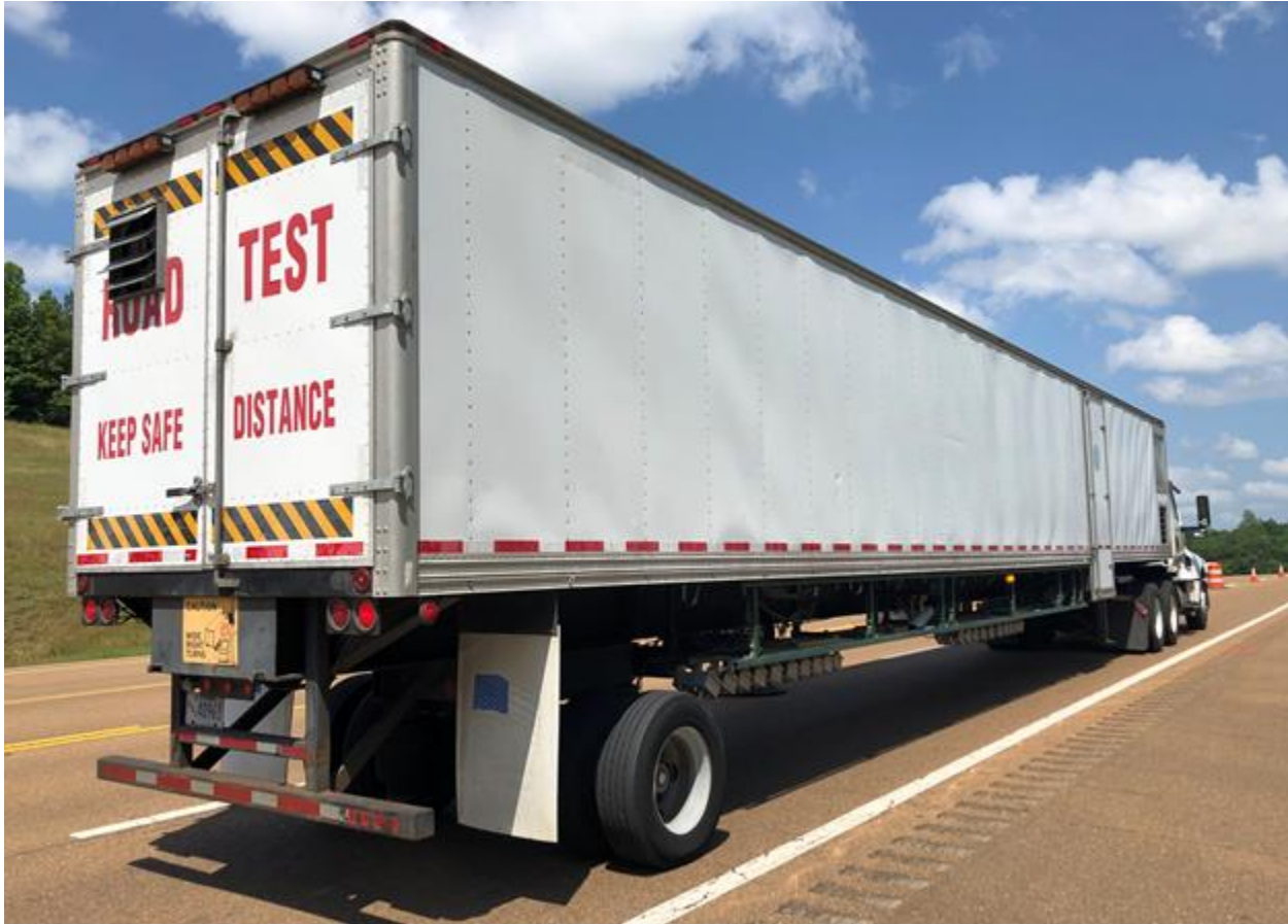
Figure 3. ARA performs structural testing with the RWD.
