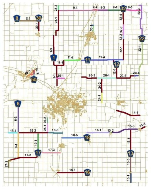
Figure 7. Champaign County PMS sections based on road, construction history, and traffic.
