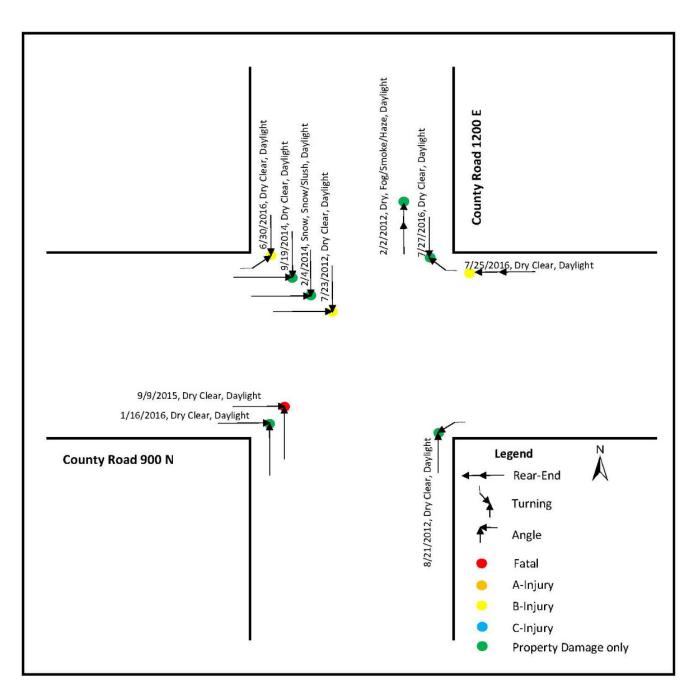
Figure 8: Collision Diagram of Crashes at intersection of County Road 1200E and County Road 900N
