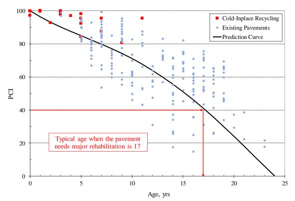
Figure 8. The typical rehabilitated pavement in Champaign County lasts 17 years before requiring its next rehabilitation.
