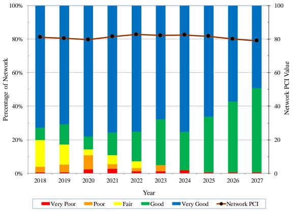
Figure 11. Predicted network condition for 2018 to 2027.
