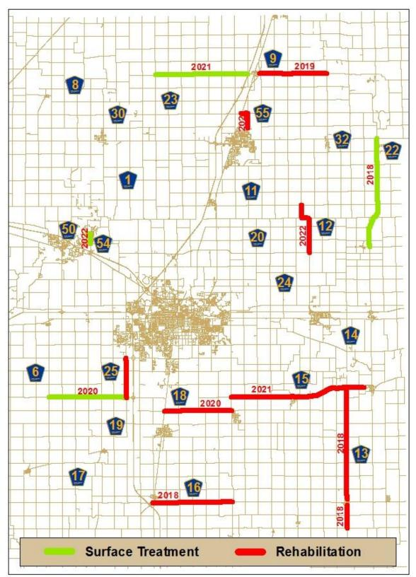
Figure 10. Rehabilitation and surface treatment plan, 2018 to 2022 (event year shown in red).
