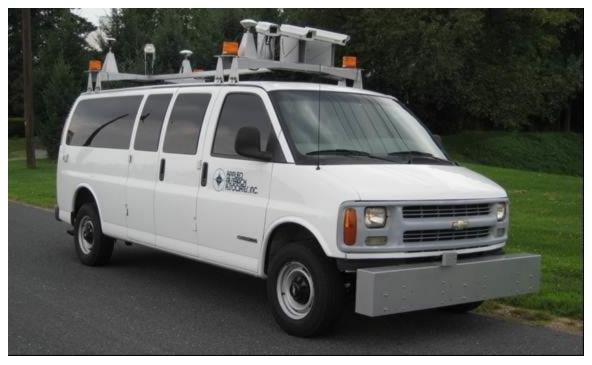
Figure 2. ARA's van-mounted camera and laser system captures high-resolution images.
