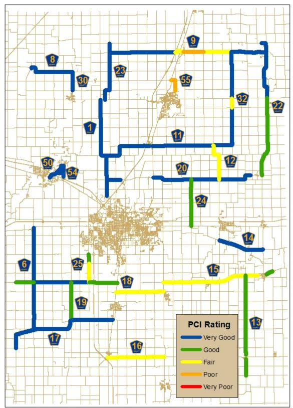
Figure 4. 2017 PCI ratings (field survey).
