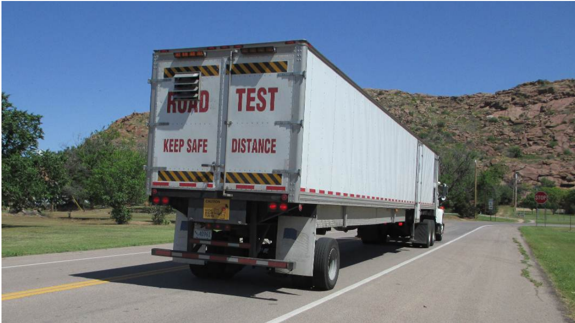
Figure 3. ARA performs structural testing with the RWD.
