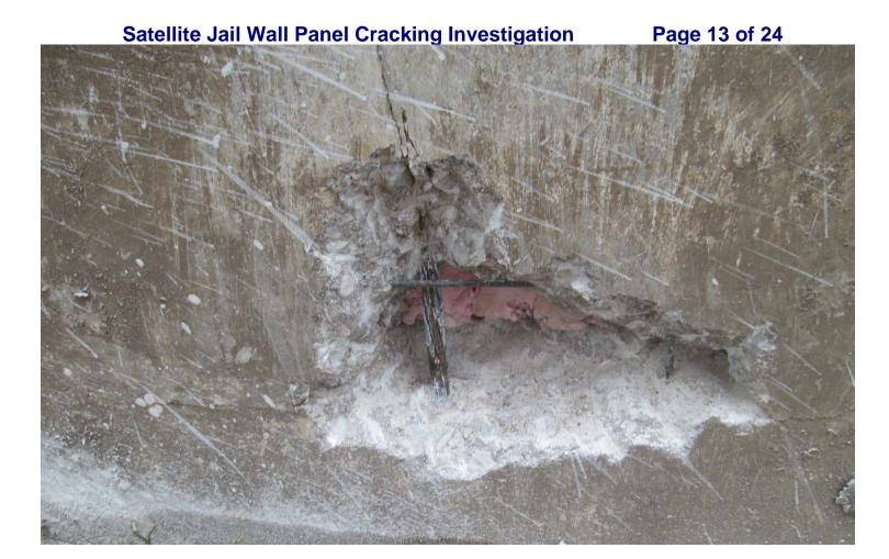
Photograph #19: The right-center strand exhibited surface corrosion.
