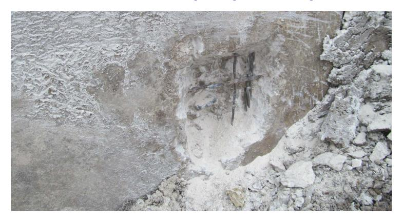
Photograph #14: The strand on the right side of the panel was corrosion free.
