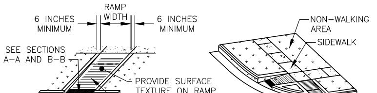
TEXTURE ON RAMP —SLOPE 1:12 (V:H) MAXIMUM TYPICAL RAMP LOCATIONS
