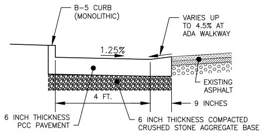
CRUSHED STONE AGGREGATION DETAIL
