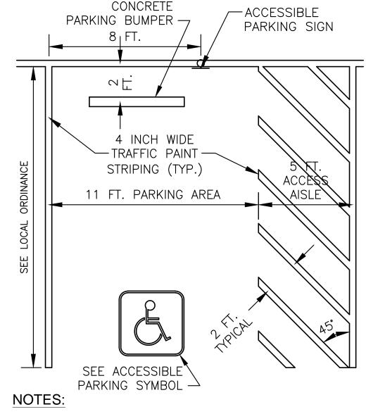
1. PARKING SPACE AND ACCESS AISLE SLOPE SHALL NOT EXCEED
