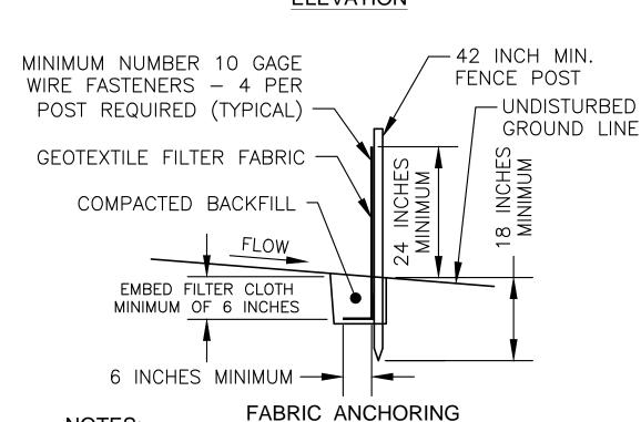
1. TEMPORARY SEDIMENT FENCE SHALL BE INSTALLED PRIOR TO ANY GRADING WORK IN THE AREA TO BE PROTECTED. THEY SHALL BE MAINTAINED THROUGHOUT THE CONSTRUCTION PERIOD AND REMOVED IN CONJUNCTION WITH THE FINAL GRADING AND SITE STABILIZATION.
